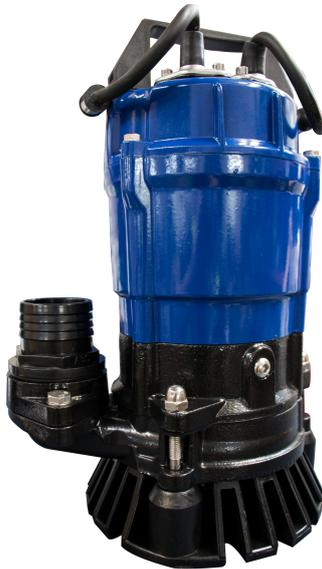
The pump is a submersible drainage pump fitted with semi vortex, eurethane coated impeller plus agitator, supplied wired and ready to install. The pump has a dual mechanical seal in oil chamber and can handle particles to 25 mm x 10mm.
