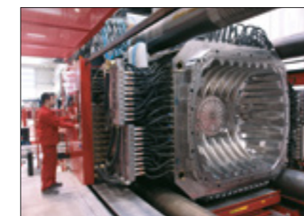
World's biggest injection moulding machine
