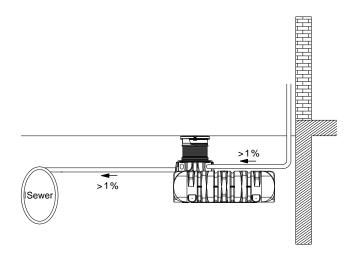
**Important:** The empty pipe must be connected to an aperture **above** the max. water level.
