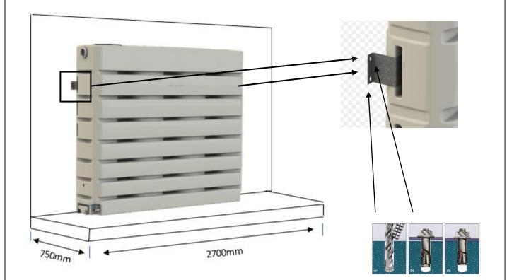
The tank should be installed on a steel reinforced concrete base capable of holding the weight of a tank full of water. Minimum recommended size of the base is 2700mm long x 750mm wide x 150mm thick.
