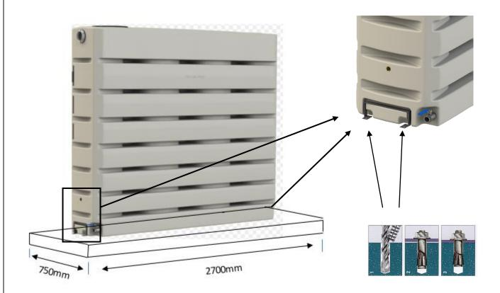
The tank should be installed on a steel reinforced concrete base capable of holding the weight of a tank full of water. Minimum recommended size of the base is 2700mm long x 750mm wide x 150mm thick.
