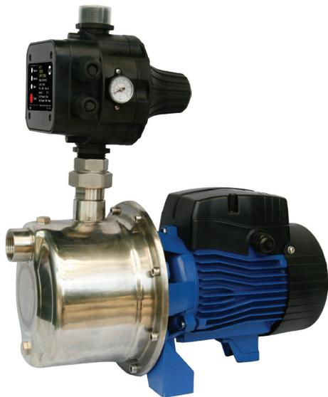
The pump is a self-priming surface mounted pressure system pump supplied with plug and play leads (IEC type). The self-priming ability provides excellent suction capacity of up to 9m. Used especially for supplying water to domestic installations.
