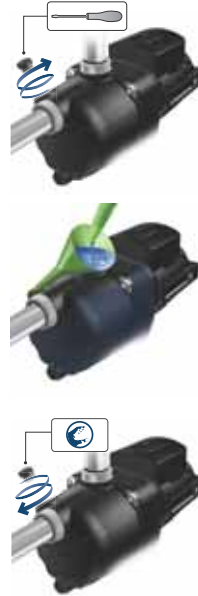
Fig. 8 Priming the pump
