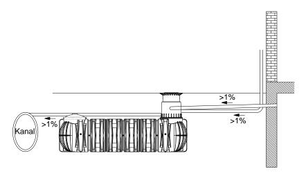
bending, to the tank with a decline. Necessary bends must be formed using 30° moulded sections.
