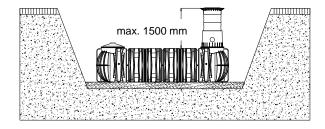
Cover heights with cast iron telescopic dome shaft (class B) in area driven over by vehicles up to 3.5 tonnes.
