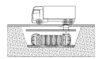
Coverage heights on installation in groundwater - the hatched area specifies the permissible immersion depth for the tank.
