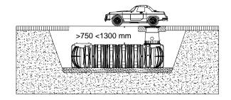
Cover heights with HGV-bearing telescopic dome shaft
