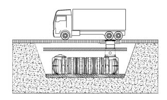
Coverage heights on installation in groundwater – the hatched area specifies the permissible immersion depth for the tank.
