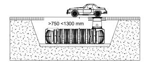
Cover heights with HGV-bearing telescopic dome shaft
