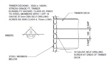
The platform must be in contact with greater than 95% of the area of the base of the tank with gaps of 5 mm(preferred) but no greater than 25mm between supports.
