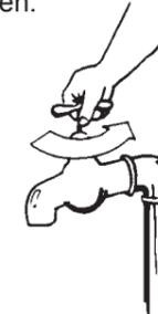
4. Prime should establish almost immediately and a strong flow of water should be evident from the outlet. Allow water to flow for 10-20 seconds to expel air then close outlet.
