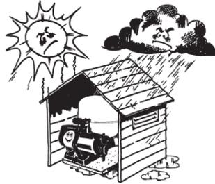
To protect your pressure system from the weather, make sure the pump house is both water proof, frost free and has adequate ventilation. The pump should be horizontally mounted on a firm base allowing for drainage, to avoid damage to flooring etc., that over time may occur from leaking pipe joints or pump seals. Do not mount the pump vertically.
