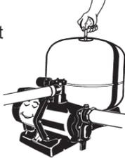
**CAUTION:** To prevent personal injury, ensure all water pressure is released from the pressure system prior to work being performed.
