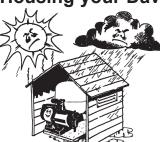
To protect your pressure system from the weather, make sure the pump house is both water proof, frost free and has adequate ventilation. The pump should be horizontally mounted on a firm base allowing for drainage, to avoid damage to flooring etc., that over time may occur from leaking pipe joints or pump seals. Do not mount the pump vertically.
