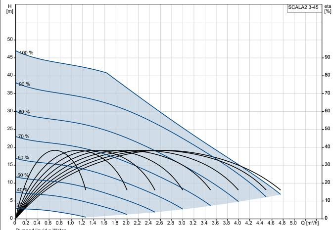
Pumped liquid = Water Liquid temperature during operation = 20 °C Density = 998.2 kg/m<sup>3</sup>
