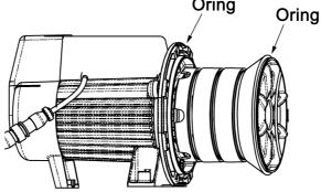
12. Assemble the pump casing with the eight casing screws to the required torque settings.
