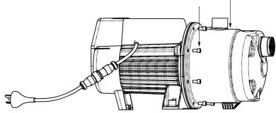
13. Replace the priming plug and oring and screw the non-return valve cartridge into the suction port, in a clockwise rotation using non specified tools (eg. a screwdriver handle, a pair of pliers, a large coin or a flat blade - 20mm wide).
