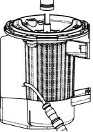
5. Fit the last stage impeller with neck ring facing you and push it down onto the mechanical seal. You will see that there are two flats running the length of the shaft and two corresponding flats in the impeller for better drive.
