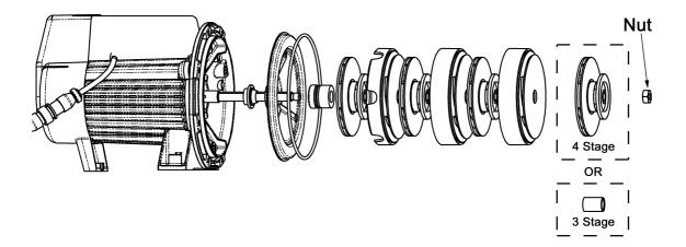
10. Locate the first stage body with the word "top" adjacent to the outlet port of the pump. Note: It is important that this stage body is assembled correctly to aid in the priming of the pump.
