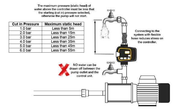
Note: The controller provides dry-run protection in both modes.
