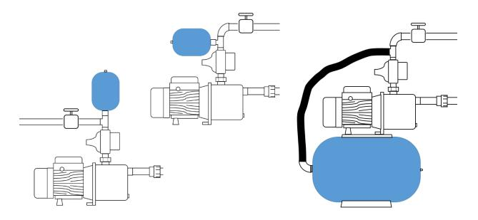
Pressure tanks should never hold more than 1/3 of its total volume as water.
