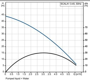
Pumped liquid = Water Liquid temperature during operation = 20 °C Density = 998.2 kg/m³
