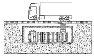
In areas where groundwater is of concern, (additionally to the requirements specified above) the permissible immersion depth for the tank in up to the shoulder of the tank.
