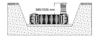
In areas with pedestrian loads only (class A installations), extension riser may be used for a maximum coverage height of 1500mm.
