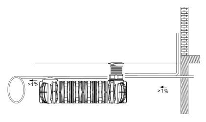
**Important:** The empty pipe must be connected to an aperture **above** the max. water level.
