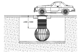
Cover heights with cast iron telescopic dome shaft (class B) in area driven over by vehicles up to 3.5 tonnes without groundwater or standing groundwater, see also 7.3.
