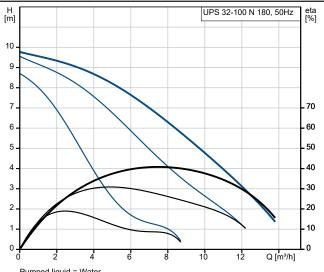
Pumped liquid = Water Liquid temperature during operation = 60 °C Density = 983.2 kg/m³
