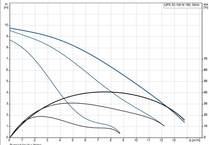
Pumped liquid = Water Liquid temperature during operation = 60 °C Density = 983.2 kg/m<sup>3</sup>
