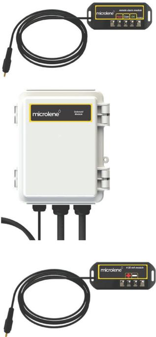
**REMOTE ALARM CONNECTION MODULE:** Allows for a connection to a remote device such as a buzzer, light, alarm system, PLC, etc., via a pair of contacts. In normal operation the OK and COM contacts will be connected, and in a fault condition (Low UV, Lamp fail, Power Fail), the Fault and COM contacts will be connected. Maximum Contact Rating is 30V / 1A (use 16-22 AWG). Order PN **DMMOD-RAM**.
