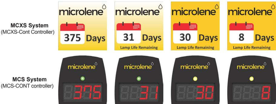
At thirty days remaining, the LED or display screen will change to a yellow caution indicator. At seven days remaining, the system will additionally repeat an audible chirp. Past the zero day threshold, the LED or display screen changes to solid red with a continuous alarm sound.
