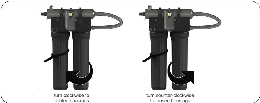
**Figure 5. Cartridge Removal**
