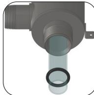
Figure 4. Quartz Sleeve Installation
