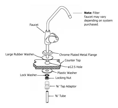
**Note:** Parts packet also contains a gasket, cone washer/olive & ¼\* Compression Nut, these are for a ¼" tube connection and are not needed for the ¾" installation.
