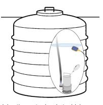
To delay the water level at which a submersible pump fitted with a float begins to operate.
