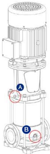
**Pump with suction lift** – check the pump data sheet for the NPSH curve.
