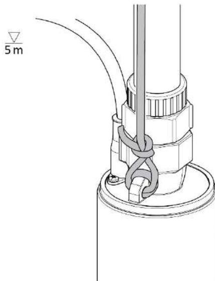
The pump must be tied with a rope to the handle before it can be submerged in the water.
