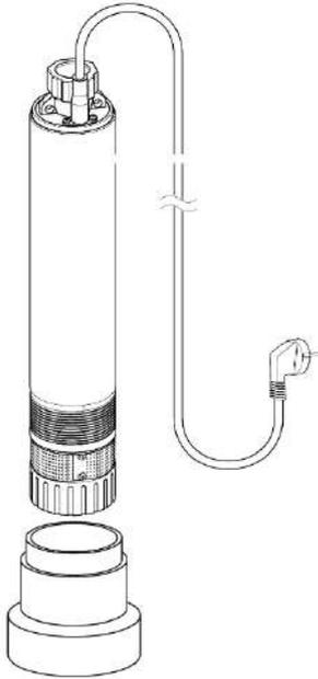
The ClayTech SLIMSUB submersible multistage pump is specially designed and manufactured for use in tanks which have a narrow or restricted opening.
