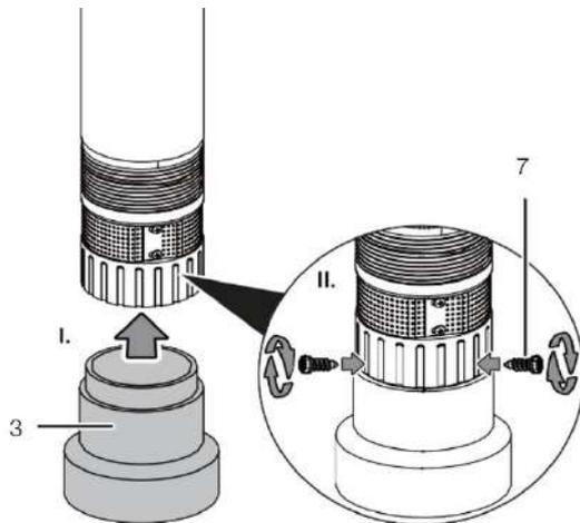
Fitting the spacer foot (3) ensures the inlet screen is raised reducing the risk of ingesting contaminants. The foot must be attached to the device prior to initial start-up.
