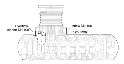
Now the prepared SUPRA®-Filter internal is installed in the tank, the elbow of the overflow from the filter is also connected now to the siphon. The inlet pipe is so to position that it is flush with the filter inlet and then finally fixed in place with the quick assembly collar.
