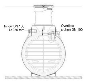
Now the prepared SUPRA®-Filter internal is installed in the tank, the elbow of the overflow from the filter is also connected now to the siphon. The inlet pipe is so to position that it is flush with the filter inlet and then finally fixed in place with the quick assembly collar.
