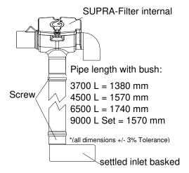
Following this a 250 mm long inlet pipe and an overflow siphon are pushed in to the Columbus underground tank until the end stop position as shown in the adjacent depiction.
