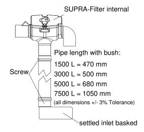
Following this a 250 mm long inlet pipe and an overflow siphon are pushed in to the Li-Lo underground tank until the end stop position as shown in the adjacent depiction.
